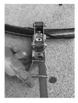
After you have completed the strip and you are holding THE RIPJACK™ by the handle, pull and hold the safety clamp's release tab (Figure 6). Open the ratchet buckle so it is completely open and flat (Figure 7).
